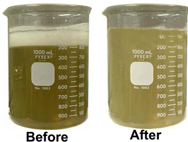
Waste Water FOG Reduction
