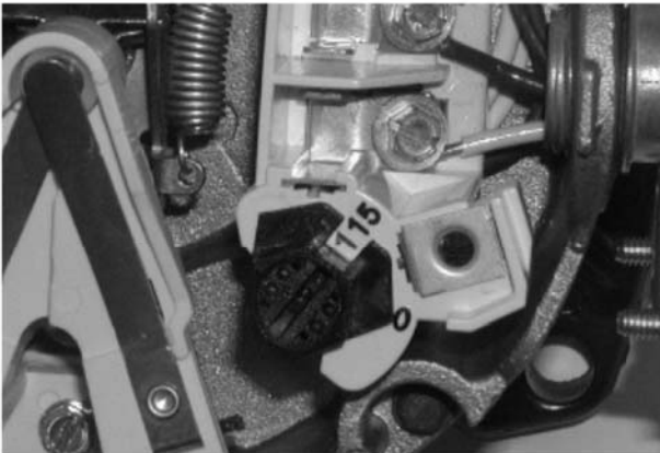
Figure 13: Motor Set for 115 Volt Operation
