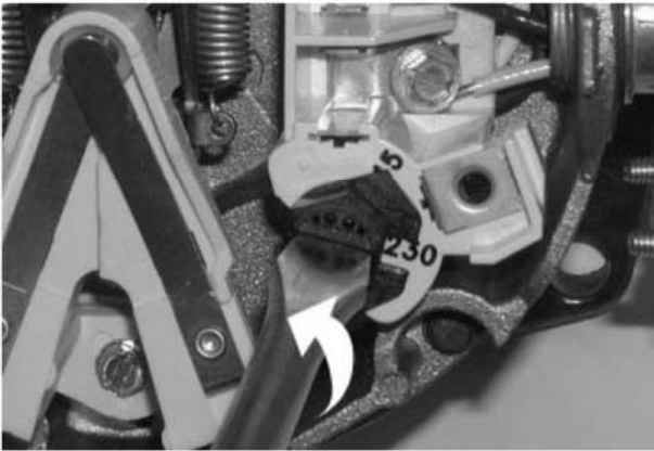
Figure 12: Changing the Voltage Setting
