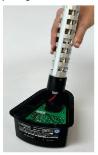
• Pull cell away from housing until lamp connector is visible.
