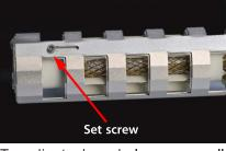
To adjust shroud, loosen small philips head screw on bottom of shroud and slide to desired position. Tighten screw.
