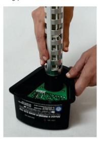
• Once housing and cell are free from mounting plate, grasp cell and turn counterclockwise while pushing down to release cell from housing.
