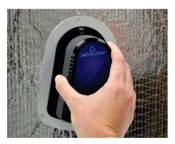
• Remove housing from unit by turning counterclockwise and pulling straight out of mounting plate.
