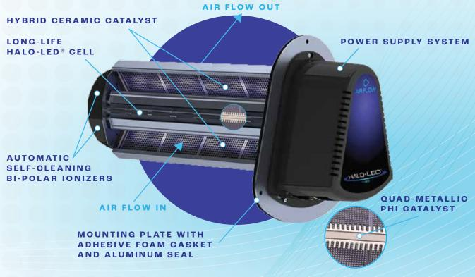
**NOTICE TO INSTALLER:** This unit must be wired in series with the blower to cycle on/off with the blower. This installation is required in order to be in compliance with new safety standards and to ensure maximum energy efficiency and LED module service life.
