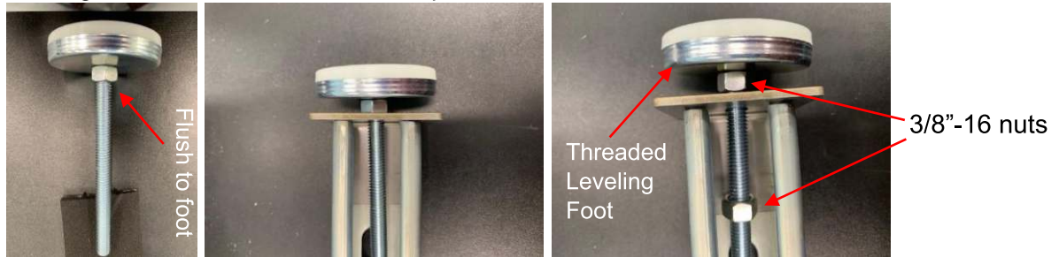
Figure (3) – Threaded Leveling Foot Attachment
