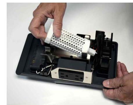
3. Remove plug from PHI Cell. Replace PHI Cell. Replace cover. Replace screws. Plug back into outlet.
